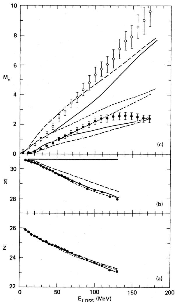
FIG. 3. Centroids of the (a) charge and (b) neutron number distributions of PLF's for the  $^{56}\text{Fe} + ^{165}\text{Ho}$  reaction at 8.5-MeV/u incident energy (Ref. 6). Note: In Ref. 6 a small correction for neutron evaporation was made to the energy loss. (c) Average multiplicity of neutrons emitted from the TLF (open circles) and PLF (filled circles) (Ref. 9). The calculations are described in the text.
