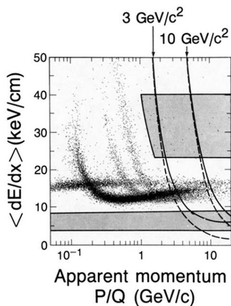
FIG. 1. Scatter plot of  $\langle dE/dx \rangle$  vs apparent momentum ( $p/Q$ ) for tracks in the data sample. The shaded regions are the search regions defined in the text. The lines are the expected ionization curves for  $Q = \frac{2}{3}$  (solid lines) and  $Q = \frac{1}{3}$  (dashed lines) particles with masses of 3 and 10  $\text{GeV}/c^2$ .
