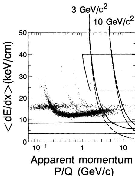
FIG. 1. Scatter plot of  $\langle dE/dx \rangle$  vs apparent momentum ( $p/Q$ ) for tracks in the data sample. The shaded regions are the search regions defined in the text. The lines are the expected ionization curves for  $Q=\frac{2}{3}$  (solid lines) and  $Q=\frac{1}{3}$  (dashed lines) particles with masses of 3 and 10 GeV/ $c^2$ .
