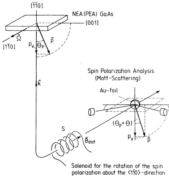
FIG. 1. Principle of the experiment: The longitudinally polarized electron beam from the GaAs(110)/(Cs,O) photocathode is deflected by 90° (giving transverse polarization) before passing through the solenoid (external magnetic field) and reaching the spin analyzer (Mott scattering).
