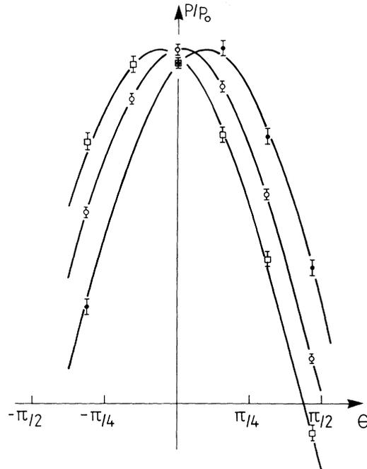
FIG. 2. Spin polarization  $P_v$  vs rotation angle  $\theta$  for three different orientations of the  $[1\bar{1}0]$  direction of the crystal with respect to the axis of the solenoid (external magnetic field  $\vec{B}_{ext}$ ). Squares,  $[1\bar{1}0]$  oriented in the apparatus as shown in Fig. 1; closed circles, after crystal rotation by 180° about  $[110]$ ; open circles,  $[1\bar{1}0] \perp B_{ext}$ .
