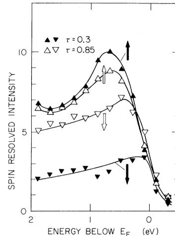
FIG. 4. Spin- and angle-resolved energy-distribution curves of Fe(100) at 31 eV photon energy for  $\tau = T/T_C=0.3$  and 0.85 (unsmoothed data).
