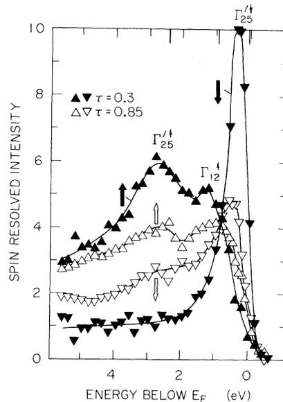
FIG. 3. Spin- and angle-resolved energy-distribution curves of Fe(100) taken at 60-eV photon energy for two different temperatures,  $\tau = T/T_C = 0.3$  and  $0.85$ , for normal emission and  $s$ -polarized light (unsmoothed data). The arrows labeling the curves refer to the direction of the spontaneous magnetization.
