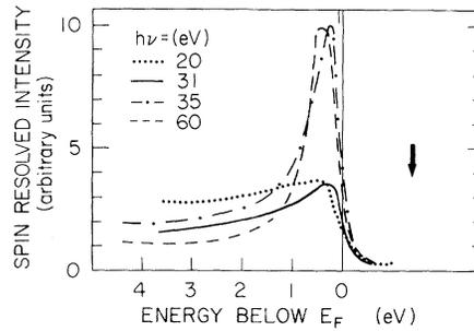
FIG. 2. Minority-spin energy-distribution curves from Fe(100) for normal emission and  $s$ -polarized light at different photon energies. The data are, at any photon energy, normalized to the maximum of  $\uparrow$ - or  $\downarrow$ -spin EDC, whichever is greater.
