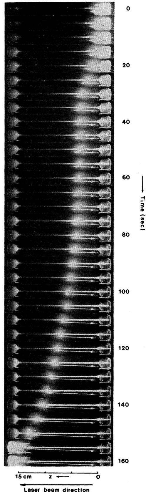
FIG. 2. Example of front propagation through the capillary cell. For  $t < 0$  the Na density is uniformly  $1 \times 10^{12} \text{ cm}^{-3}$ . At  $t = 0$  the laser beam is admitted; the laser polarization is linear, the intensity is  $3 \text{ W cm}^{-2}$ , and the frequency is tuned in the red Na  $D_2$  Doppler wing,  $\nu_L = \nu_{F=2} - 0.85 \text{ GHz}$ .
