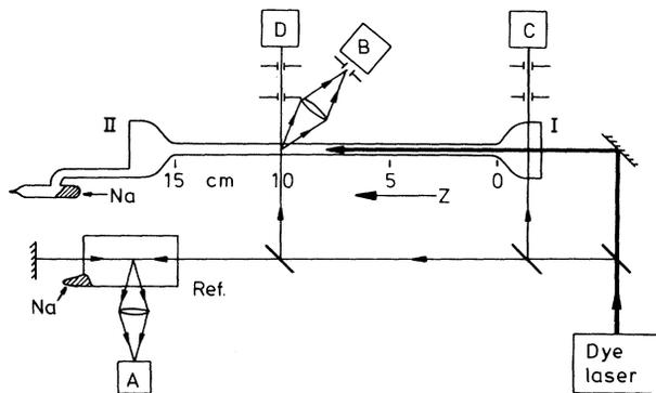
FIG. 1. Experimental setup; the capillary cell has been filled with 10 Torr of Ar (at 300 K). *A*, *B*, *C*, and *D* are photodiodes. Lamb dips in the Na *D* fluorescence spectrum from a reference Na cell (without buffer gas) are used for frequency calibration.
