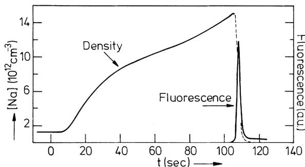
FIG. 3. Na density in the capillary cell and Na fluorescence from the capillary cell, both at  $z = 10$  cm (see Fig. 1), as a function of time during propagation of the front. The laser beam is admitted at  $t = 0$ . The Na density could not be measured during passage of the fluorescent spot; a dashed line has been drawn to guide the eye. Laser polarization, intensity, and frequency are as in Fig. 2.
