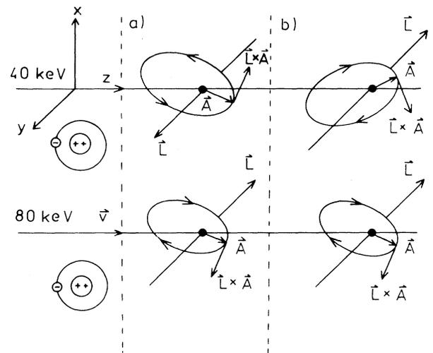
FIG. 2. "Classical" orbits of the coherently excited electron (see text); (a) model suggested by the CDW-PCI approximation; (b) possible alternative also consistent with the data of Ref. 1. All orbits lie in the  $x$ - $z$  plane.
