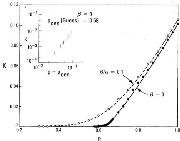
FIG. 1. Bulk moduli vs  $p$  for the cases when the force is purely central ( $\beta=0$ ), and when the noncentral force is small ( $\beta/\alpha=0.1$ ), for the 2D triangular lattice of 946 nodes. A strong crossover is observed near  $p_{\text{cen}}$  in the latter case. Inset shows one  $\log K$  vs  $\log(p - p_{\text{cen}})$  plot.
