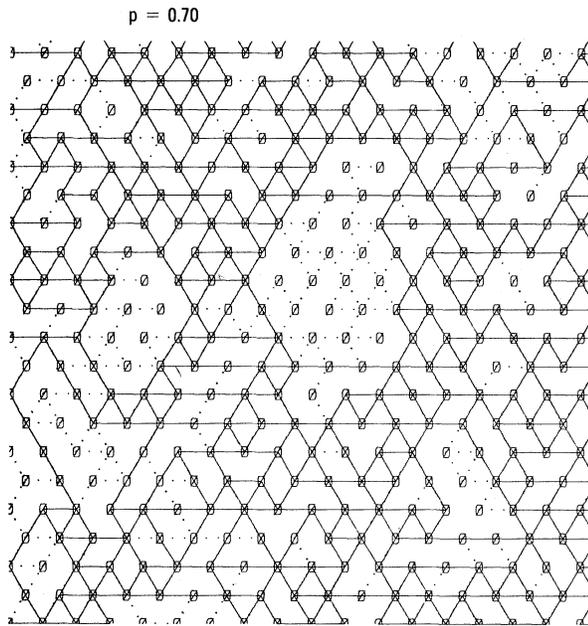
FIG. 2. Simulation of displacements of a 2D triangular lattice subjected to a hydrostatic pressure. The occupied bonds that stretched or shrank are shown by the solid lines and other occupied bonds by dotted lines. The rigid elastic backbone is given by the connected network of solid bonds. For clarity only a small portion of the network is shown.
