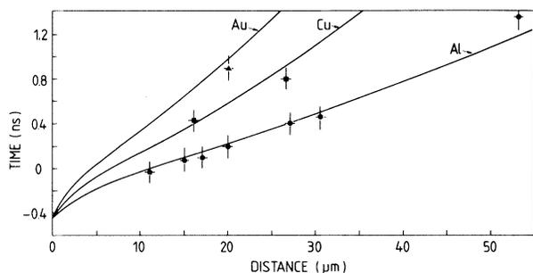
FIG. 3. Experimental points and calculated curves of shock-wave propagation in space-time coordinates for a maximum driving pressure of 3 TPa (zero time with respect to the peak of the laser pulse). The average laser energy is 8 J in 450-ps FWHM on 50- $\mu\text{m}$ -diam spot at half energy at 0.26- $\mu\text{m}$  wavelength.
