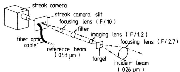
FIG. 1. Schematic configuration of the experimental setup for measurement of laser-induced shock-wave transit time through a thin target.
