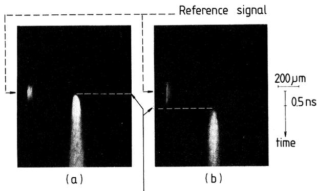
FIG. 2. Streak-camera records of luminosity produced by the emergence of a shock wave at the rear face of a metal target irradiated by a 450-ps-FWHM laser pulse on a 50- $\mu\text{m}$ -diam focal spot at half energy,  $4.5 \times 10^{14} \text{ W/cm}^2$  incident energy. (a) 15- $\mu\text{m}$ -thick aluminum foil, (b) 16- $\mu\text{m}$ -thick copper foil.
