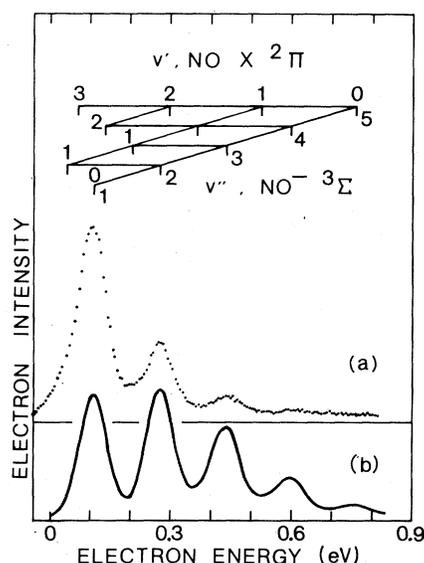
FIG. 2. (a) Energy spectrum of electrons detached in 2.5-keV  $H^-$ - $NO$  collisions observed at  $90^\circ$ . (b) Calculated energy spectrum of electrons autodetached from the  $NO^-$   $^3\Sigma$  resonance.
