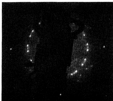
FIG. 2. LEED pattern of a potassium monolayer on copper (001) for \theta = 0.37 , at incident electron energy of 53 eV, and substrate temperature of 330 K.
