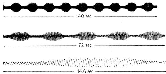
FIG. 5. The response of a height transducer placed at the midpoint of the oscillating solitons of Fig. 4. The lowest trace covers the complete sequence of Fig. 4. The frequency of the envelope is  $2\nu/(156 \pm 0.5) = 0.068$  Hz. The upper traces are recorded at successively slower paper speeds.
