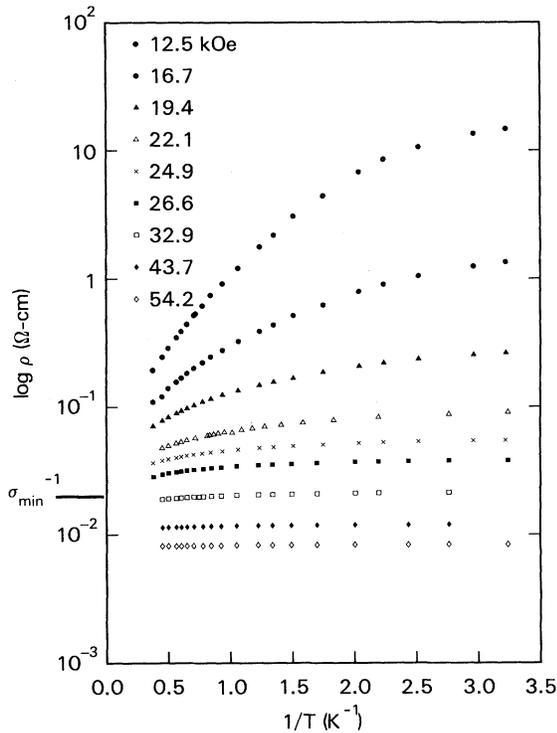
FIG. 1. Temperature dependence of magnetoresistivity of  $Gd_{3-x}V_xS_4$  sample No. 1. An estimate for  $\sigma_{\min}^{-1}$  is indicated and discussed in the text.
