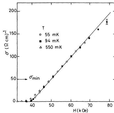
FIG. 3. Magnetic field dependence of conductivity of  $Gd_{3-x}V_xS_4$  sample No. 2 at  $T=55, 94,$  and  $550$  mK. The fitted line obeys the equation
