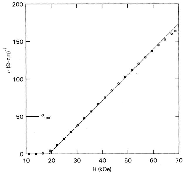
FIG. 2. Magnetic field dependence of conductivity of  $Gd_{3-x}V_xS_4$  sample No. 1 at  $T=300$  mK. The fitted line obeys the equation
