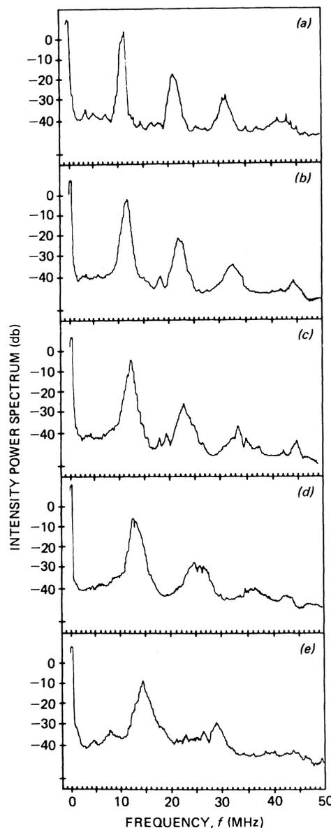
FIG. 4. Broadening of pulsation spectral peaks (resolution 100 kHz) with increasing discharge current for 175-mTorr Xe and no helium [ $\gamma = (2.0 \pm 0.1) \times 10^7 \text{ s}^{-1}$ ;  $\kappa = (3.3 \pm 0.5) \times 10^8 \text{ s}^{-1}$ ]. Discharge currents and relative average power outputs are (a) 0.83 mA, 6.2; (b) 0.91 mA, 6.7; (c) 1.0 mA, 7.3; (d) 1.2 mA, 8.3; (e) 1.5 mA, 9.5.
