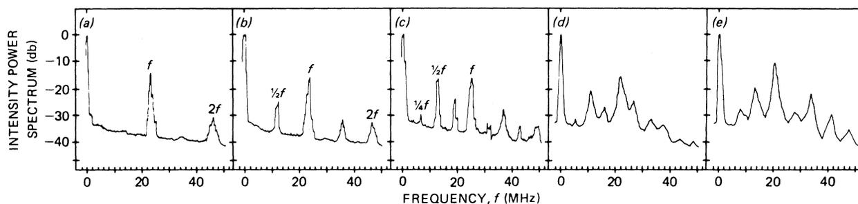
FIG. 2. Power spectra (resolution 1 MHz) of laser output intensity for different detunings in the expanded scale region of Fig. 1 showing period-doubling route to chaos. Spectra are taken from (a) to (e) as samples from the P1, P2, P4, C4, and C3 regions of Fig. 1.
