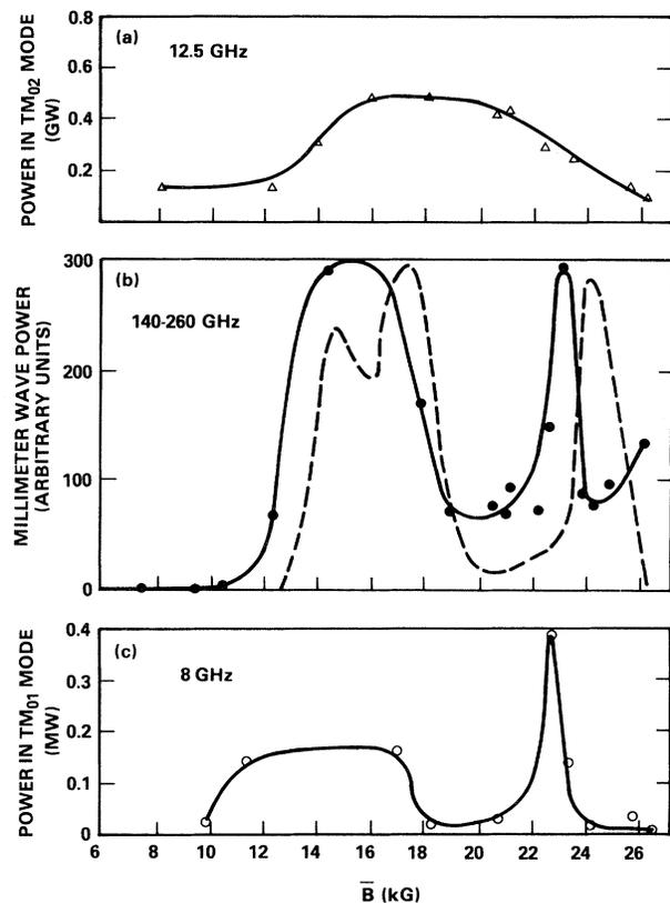
FIG. 3. Magnetic signatures of power emitted at various frequencies from two-stage BWO-FEL experiment. (a) BWO emission ( $TM_{02}$ ) at 12.5 GHz vs  $\bar{B}$ . (b) High-frequency FEL emission at  $f > 140$  GHz vs  $\bar{B}$ . Dashed line is magnetic signature of high-frequency emission from an FEL with magnetostatic wiggler. (c) Low-frequency FEL emission ( $TM_{01}$ ) at 8 GHz vs  $\bar{B}$ .
