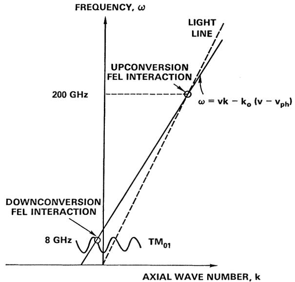
FIG. 4. Dispersion relations for FEL interaction ( $k_0 = -1.2 \times 10^2$  m<sup>-1</sup>,  $v_{ph} = -7 \times 10^8$  m/sec).
