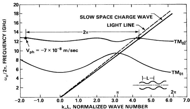
FIG. 2. Dispersion relations for BWO interaction showing coupling of the slow space-charge wave to the  $TM_{02}$  mode of the rippled-wave waveguide. The position of the fundamental  $TM_{02}$  BWO emission is indicated  $2\pi$  away from the normalized interaction wave number.
