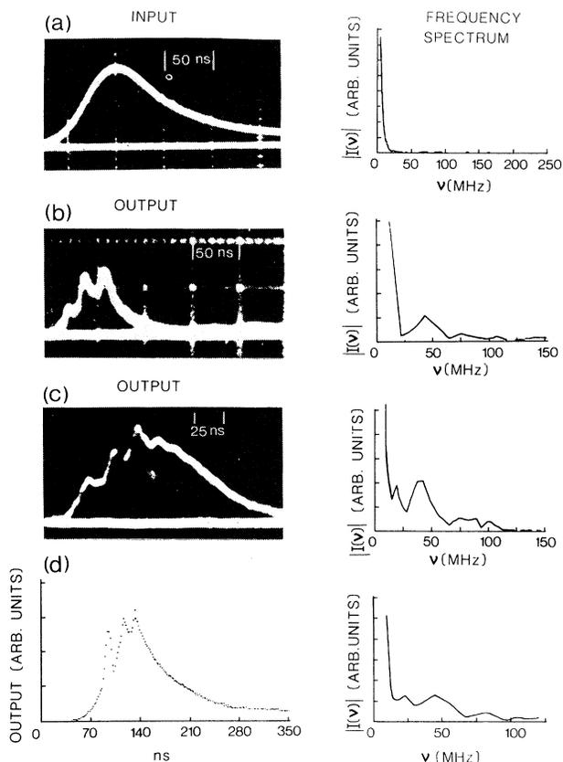
FIG. 2. Sample oscilloscope traces of (a) the pump signal and (b)–(d) the ring-cavity signal, together with their frequency spectra; obtained from digitized traces as shown in (d).
