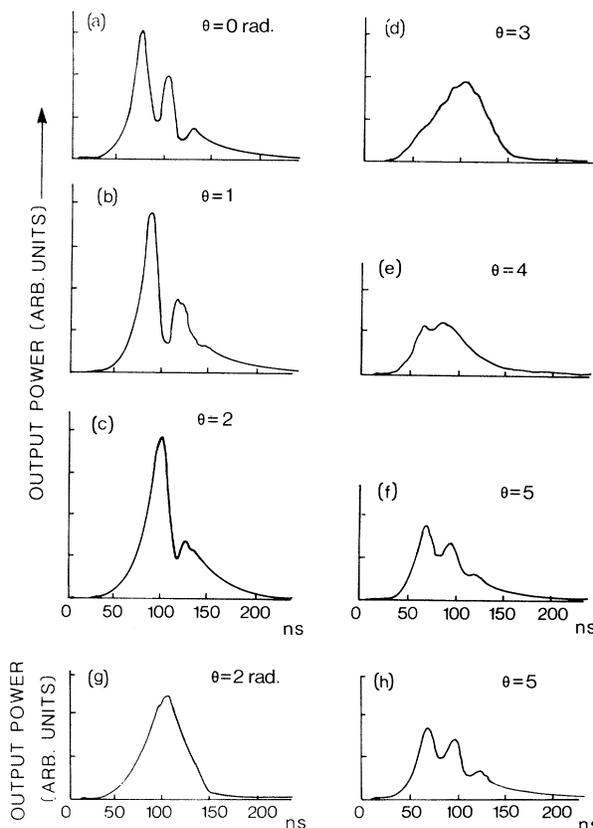
FIG. 4. Numerically determined ring-cavity signals for various cavity tunings using Fig. 2(a) as the pump signal. ( $\alpha L = 3$ ,  $kt_R = 5$ ,  $Kt_R = 0.1$ ,  $|e|_{\text{max}}^2 = 0.9$ .)
