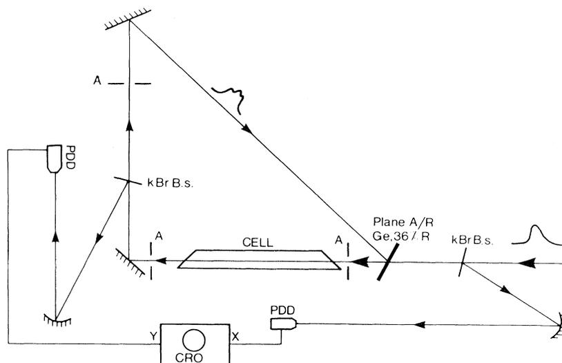
FIG. 1. Schematic diagram of ring-cavity system. B.s.: beam splitter; PDD: photon-drag detector; A/R: anti-reflection coated.
