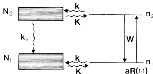
FIG. 3. Kinetic model for  $\text{NH}_3$  absorption. Radiative coupling is represented by continuous lines and collisional relaxation (both rotational and vibrational) by wavy lines.
