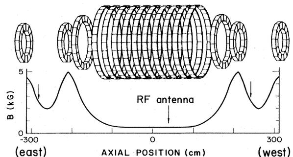
FIG. 1. The axisymmetric coil set and axial field strength profile. The locations of the rf heating antennas are indicated by the arrows. In the plugs the antenna is a straight copper rod (Ref. 3) 6 cm from the axis and in the central cell the antenna is a one-half-turn copper strap ( $r=22 \text{ cm}$ ). No Faraday shielding is used here.
