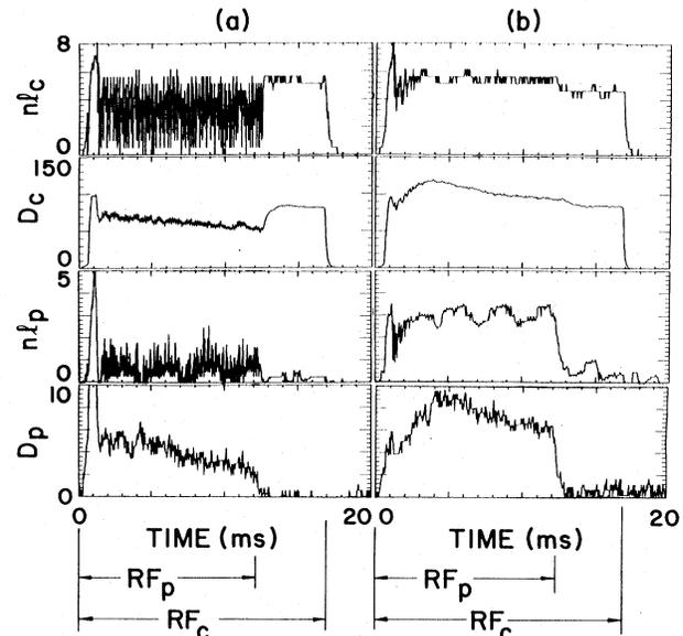
FIG. 3. East plug and central-cell line density ( $n/l$ ,  $10^{13}$  cm $^{-2}$ ) and diamagnetism [ $D = n(T_e + T_i)/B$ ,  $10^{10}$  eV/cm $^3$  G] for two shots with different plug field strengths and fixed rf frequencies,  $f_p = 2.95$  MHz. (a) Plug midplane field is 1922 G, field at the plug antenna is 2458 G. (b) Plug midplane field is 1715 G, field at the plug antenna is 2179 G.
