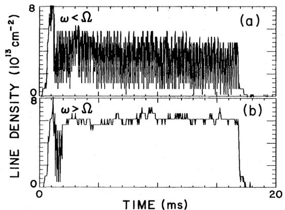
FIG. 2. The central-cell line density for single-cell operation measured with a 4-mm microwave interferometer. The vacuum field strength was varied between shots with the rf frequency fixed at  $f = 680$  kHz. (a)  $B = 444$  G, (b)  $B = 442$  G. From the calibration and resolution of the coil current meters the absolute magnitude of the field is known  $\pm 2\%$  but the change in field strength is known to be  $2 \pm 0.5$  G.
