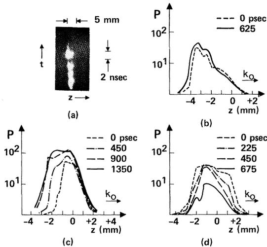
FIG. 2. (a) Typical streak image at 15-nsec full frame. (b)–(d) Microdensitometer scans of streak images of three shots showing relative scattered power  $P \propto (\bar{n}/n_0)^2$  vs  $z$  at various times during the pulse. One acoustic period is  $\approx 100$  psec. The CO<sub>2</sub> best focus is at  $z = 0$ .
