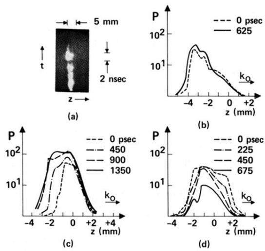
FIG. 2. (a) Typical streak image at 15-nsec full frame. (b)–(d) Microdensitometer scans of streak images of three shots showing relative scattered power  $P \propto (\tilde{n}/n_o)^2$  vs  $z$  at various times during the pulse. One acoustic period is  $\approx 100$  psec. The  $\text{CO}_2$  best focus is at  $z=0$ .
