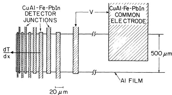
FIG. 1. Sample configuration. Note the two different length scales.
