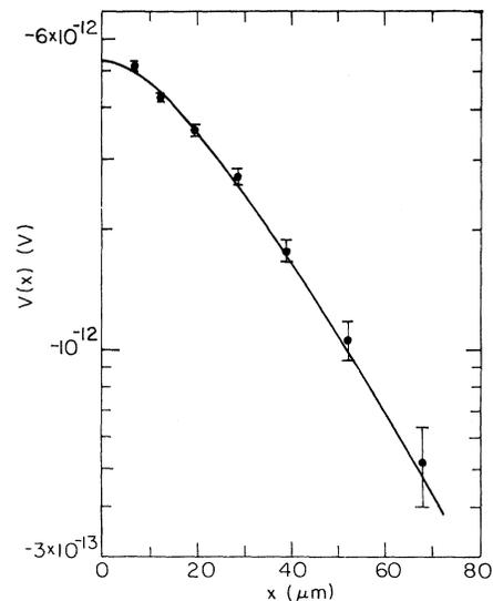
FIG. 2. Measured values of  $V(x)$  for sample 1 ( $T_s = 0.978T_c$ ,  $dT/dx = 28.1$  K m<sup>-1</sup>) in presence of temperature gradient. Solid line is from Eq. (4) with  $\lambda_{Q^*} = 14.5$   $\mu\text{m}$ ,  $\lambda_T = 19$   $\mu\text{m}$ , and  $S^S = -3.0 \times 10^{-8}$  V K<sup>-1</sup>.
