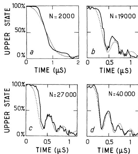
FIG. 2. Evolution of the normalized upper-level population  $N_e/N$  as a function of time, for increasing total atom number  $N$ . Solid line: experiment; dotted line: theoretical calculation. (a) Overdamped regime; (b)–(d) self-induced ringings with increasing frequency. Note the different time scales of (a) and (b)–(d).
