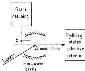
FIG. 1. Sketch of experimental arrangement. The millimeter-wave cavity is made of two copper spherical mirrors of 60-mm radius of curvature and 27-mm-diam aperture, in the cofocal geometry (60 mm between mirrors). The measured cavity finesse is 3200 at 82 GHz.
