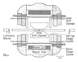
FIG. 1. The high resolution spectrometer (HRS).
