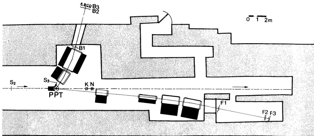
FIG. 1. Layout of the experiment. The unpolarized proton beam scattered in the vertically polarized-proton target (PPT) and the elastic events were detected by the  $F$  and  $B$  scintillation counter hodoscopes. The  $N$  and  $K$  counters were intensity monitors, while  $S_2$  and  $S_3$  were segmented wire ion chambers which monitored the beam's position, size, and angle.
