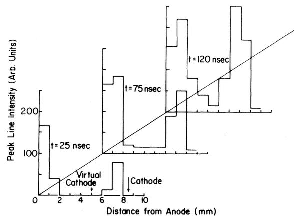
FIG. 2. Peak line intensity (PMT signal of channel 1 with  $\lambda = 4861.5 \text{ \AA}$ ) as a function of distance from anode at different times. Spatial resolution  $\approx 1$  mm.
