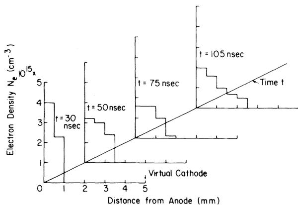
FIG. 3. Electron density as a function of distance from anode at different times.  $V_D=400$  kV,  $J_i=120$  A/cm<sup>2</sup>,  $B/B^*=1.5$ .
