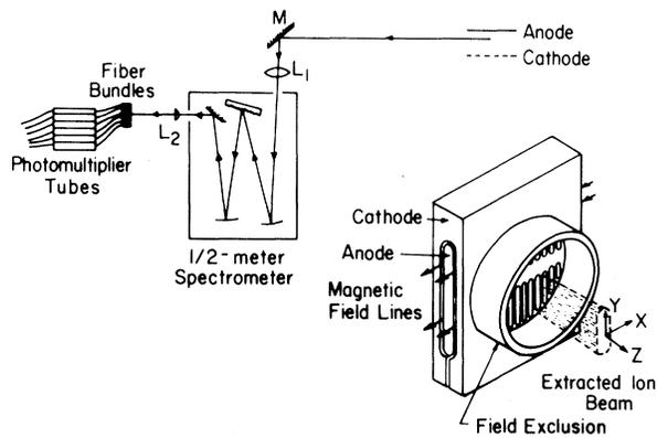
FIG. 1. Schematic diagrams of the optical setup and the "racetrack"-diode assembly.
