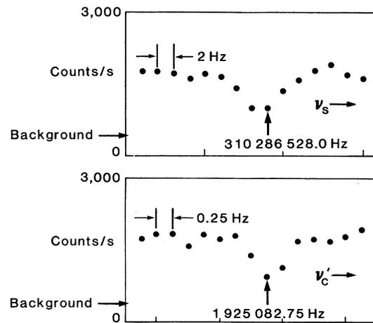
FIG. 2. Example cyclotron ( $\nu_c'$ ) and spin ( $\nu_s$ ) resonances. These curves were taken nearly simultaneously by the technique described in the text.  $B_0 \cong 1.134 \text{ T}$ ,  $\nu_z \cong 215 \text{ kHz}$ .
