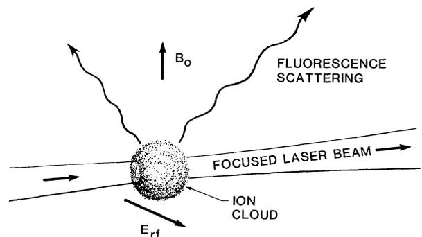
FIG. 1. Basic technique. A small sample of ions is confined by static magnetic and electric fields (not shown). A laser beam is focused onto the sample and the fluorescence scattering is observed. When the cyclotron motion is excited by an externally applied electric field ( $\vec{E}_{rf}$ ) the ion orbits increase in size which results in a decrease in fluorescence.
