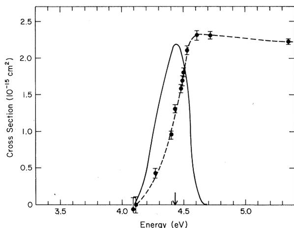
FIG. 4. Threshold cross section for  $\text{Mg}^+(3s \rightarrow 3p)$  excitation (experimental points and dotted curve). Solid line is first derivative representing the mirror image of electron beam energy distribution. Arrow indicates excitation threshold energy.
