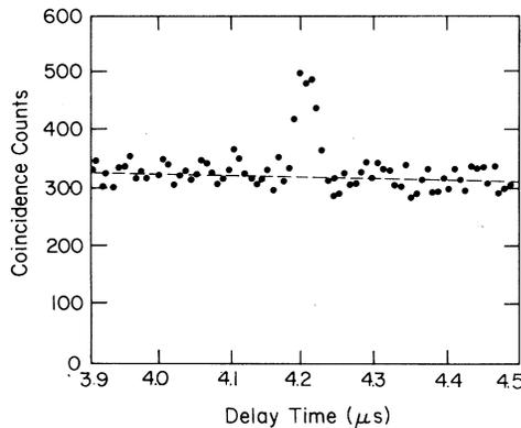
FIG. 3. Dielectronic recombination coincidence spectrum; dashed line is least-squares fit to background.
