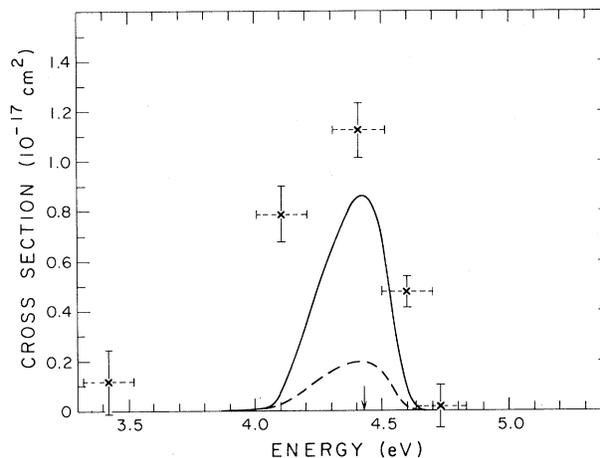
FIG. 5. DR cross section vs energy for  $e + \text{Mg}^+$ ; crosses, experiment; dashed curve, convolution of theory (Ref. 23) for  $n \leq 64$  with experimental electron energy distribution; solid curve, same as dashed curve, including all  $n$ . Arrow indicates excitation threshold energy. Bars are relative uncertainty only. The absolute uncertainty in cross section is  $\pm 58\%$  (see text).
