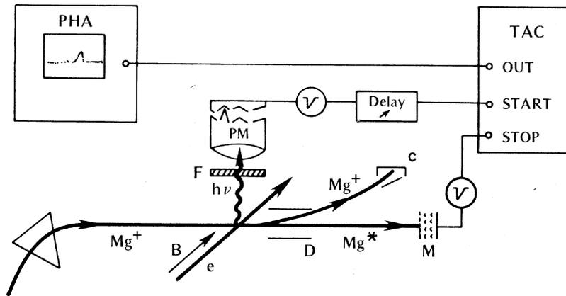
FIG. 2. Schematic representation of the experimental apparatus.
