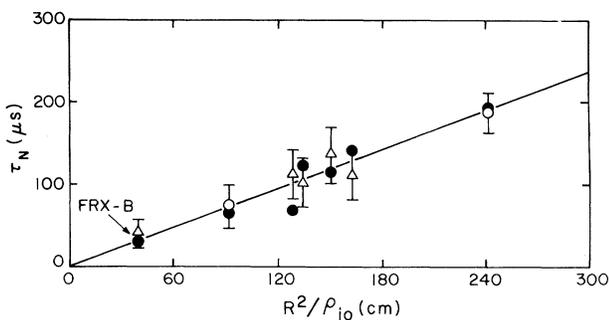
FIG. 3. Scaling of particle confinement time,  $\tau_N$ , with  $R^2/\rho_{i0}$ ; open circles, from end-on holography; triangles, from side-on interferometer and  $r_{\Delta\phi}$  axial profile; and solid circles, predictions from Tuszewski-Linford lower-hybrid transport model. The solid straight line represents an empirical fit to the experimental data.
