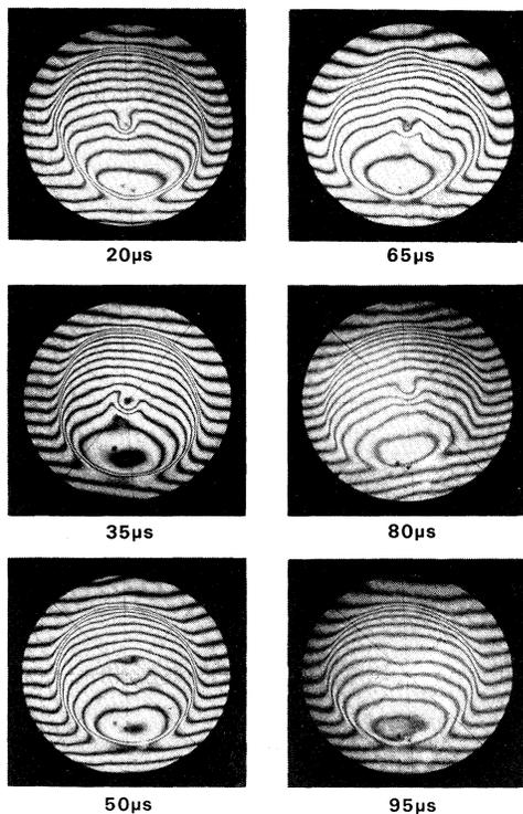
FIG. 1. Time sequence of interferograms taken during the FRC quiescent phase. Each interferogram was recorded separately on a single discharge, and the diameter of the interferometer field of view was 30 cm.
