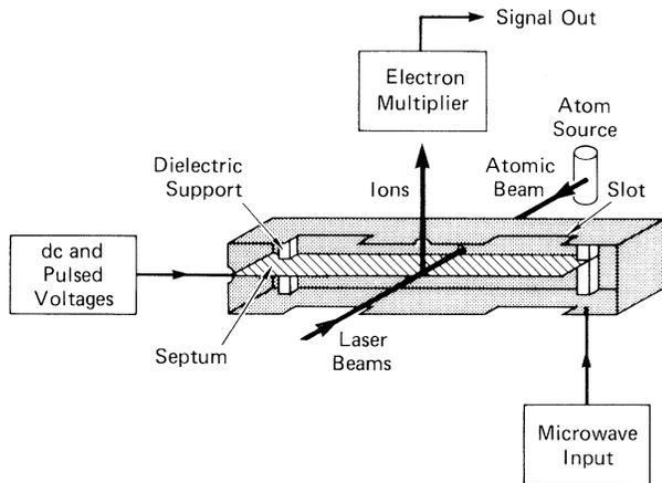
FIG. 2. Cut-away view of the microwave cavity (not to scale). The copper septum bisects the height of the cavity. Two holes of diameter 1.3 mm are drilled in the sidewalls to admit the collinear laser and Na atomic beams, and a 1-mm hole in the top cavity allows Na<sup>+</sup> resulting from the field ionization of Na to be extracted.
