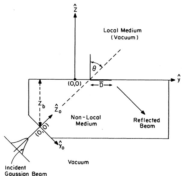
FIG. 1. The laser beam is incident from vacuum at the lower left surface, and propagates to the upper reflecting interface where it is totally internally reflected since  $\theta \sim \theta_c$ . This is the “Goos-Hänchen” geometry with the “model crystal” cut so as to permit normal incidence at the lower left surface (see Ref. 3).
