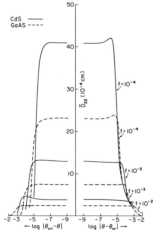
FIG. 2. Goos-Hänchen shift  $\bar{D}_{22}$  plotted against  $\log(|\theta - \theta_{2c}|)$ . Material parameters used (see Ref. 4): for CdS,  $\epsilon_\infty = 8.0$ ,  $\hbar\omega_0 = 2.55$  eV,  $m^* = 0.9m_e$ ,  $4\pi\alpha_0 = 0.0125$ , and  $\Gamma/2\omega_0 = 10^{-5}$ . For GaAs,  $\epsilon_\infty = 12.55$ ,  $\hbar\omega_0 = 1.55$  eV,  $m^* = 0.6m_e$ ,  $4\pi\alpha_0 = 0.0013$ , and  $\Gamma = 0.1$   $\text{cm}^{-1}$ .
