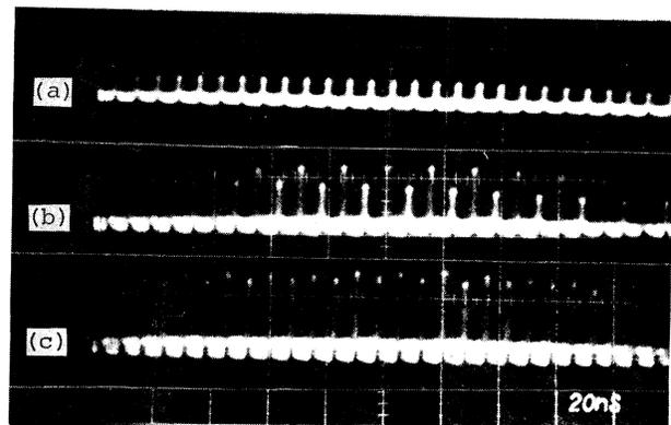
FIG. 3. Oscilloscope traces of the center part of the output envelope from the ring cavity for respective input power levels of (a), (b), and (c) in Fig. 2. Vertical gain of the oscilloscope in (c) is reduced by a factor of 2 from that in (a) and (b). Horizontal scale is 20 ns/div.
