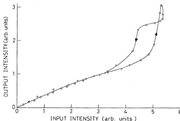
FIG. 6. Output vs input intensity in the case of the oscilloscope trace of Fig. 5(a) when the ring cavity is lengthened by 6 mm.
