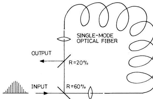
FIG. 1. Schematic diagram of the experiment.
