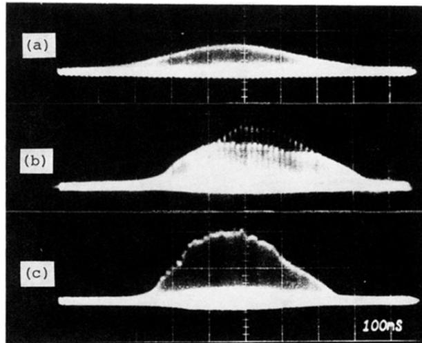
FIG. 2. Oscilloscope traces of the output from the ring cavity. The power levels of the input to the cavity are 50, 160, and 300 W for (a), (b), and (c), respectively. Horizontal scale is 100 ns/div.
