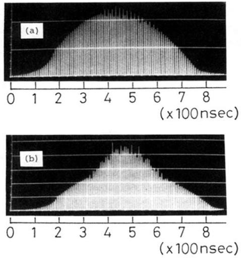
FIG. 4. Computer simulations of the output from the ring cavity: (a) period-two state where  $\varphi_0 = \pi/2$ ,  $B = 0.4$ ,  $A^2B = 1.3$ , and (b) chaos where  $\varphi_0 = \pi/2$ ,  $B = 0.4$ ,  $A^2B = 2.5$ .
