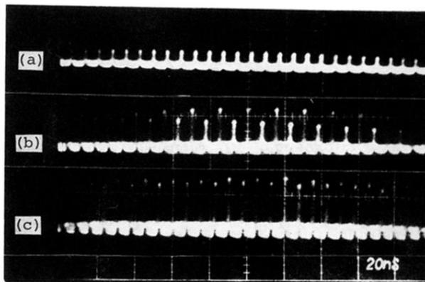
FIG. 3. Oscilloscope traces of the center part of the output envelope from the ring cavity for respective input power levels of (a), (b), and (c) in Fig. 2. Vertical gain of the oscilloscope in (c) is reduced by a factor of 2 from that in (a) and (b). Horizontal scale is 20 ns/div.
