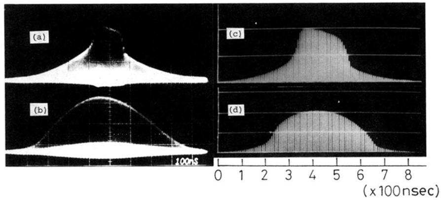
FIG. 5. (a), (b) Two examples of oscilloscope traces of the output from the ring cavity (the peak input power is 160 W), and (c), (d) their computer simulations ( $B = 0.4$ , and  $A^2B = 1.1$ ), when the cavity is lengthened by 6 mm.  $\varphi_0$  is different between (a) and (b), and between (c) and (d).
