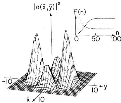
FIG. 3. The steady-state wave front  $|a(\bar{x}, \bar{y})|^2$  at the output mirror  $M2$  after  $n = 100$  passes. The off-axis electron beam with  $\Delta\bar{y} = 1.0$  has distorted the steady-state wave front into four distinct peaks. The peak optical field  $|a|_{\max} = 15$  and the wave-front energy is increased to a final value of  $E(100) = 1100$ .
