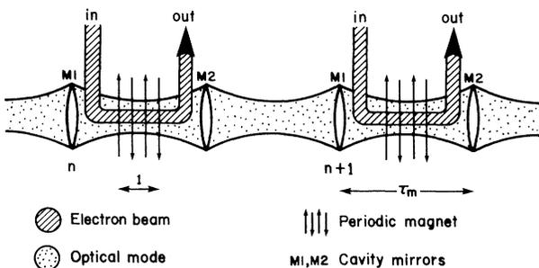
FIG. 1. The resonator cavity unfolded in time to follow the evolution of the optical wave front. In this view the mirrors  $M1$  and  $M2$  act as lenses to focus the wave front back to the mode axis. The wave front is amplified by a new electron beam on each pass through the laser's undulating magnetic field.
