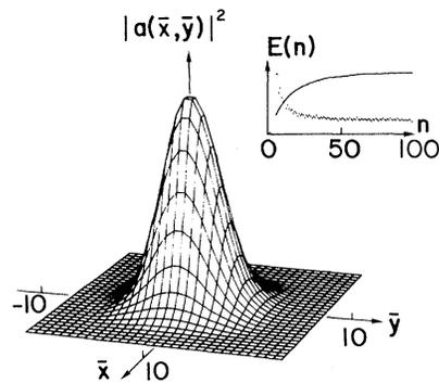
FIG. 2. The steady-state wave front  $|a(\bar{x}, \bar{y})|^2$  at the output mirror  $M2$  after  $n=100$  passes resembles the  $TEM_{00}$  cavity mode. The wave-front energy  $E(n)$  (inset curve) has increased to a final value of  $E(100) = 2600$ .
