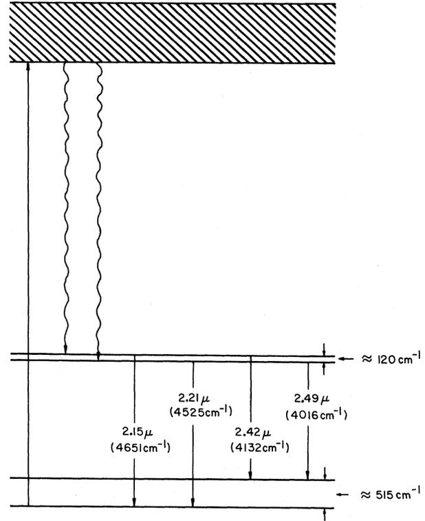
FIG. 1. Energy level diagram of trivalent uranium in calcium fluoride based on the paper by Galkin and Feofilov. Broad-band pumping light applied in the blue and green visible spectrum causes transitions to excited bands, one of which is depicted in the figure. These pumping transitions are followed by rapid, non-radiative transitions to the two metastable levels shown.
