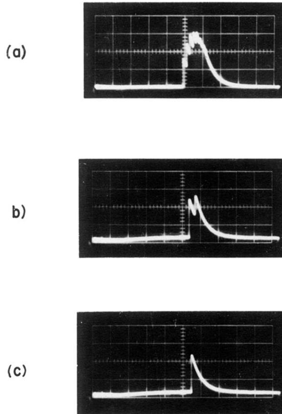
FIG. 3. Relaxation oscillations at varying pump power levels. The time scale is  $100 \mu\text{sec}/\text{division}$ . Trace (a) shows the maser output with pump power about 1.5% above threshold. Traces (b) and (c) are taken at powers barely above threshold.
