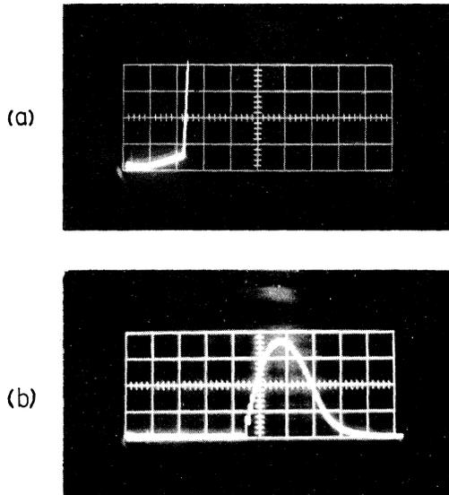
Fig. 2. (a) Detector response above threshold showing the onset of oscillation after 450  $\mu\text{sec}$ . A filter with a bandwidth of 0.1 micron and centered at 2.5 microns is inserted before the detector. The sweep speed is 200  $\mu\text{sec}/\text{division}$ . (b) Detector response with the conditions as in 2(a) except that the oscilloscope gain is reduced by a factor of 500 and the sweep speed is 100  $\mu\text{sec}/\text{division}$ .
