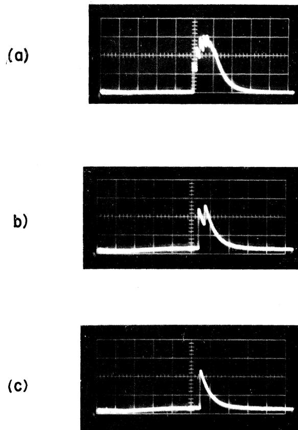
FIG. 3. Relaxation oscillations at varying pump power levels. The time scale is 100  $\mu\text{sec}/\text{division}$ . Trace (a) shows the maser output with pump power about 1.5% above threshold. Traces (b) and (c) are taken at powers barely above threshold.
