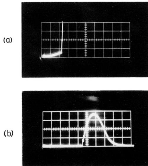
Fig. 2. (a) Detector response above threshold showing the onset of oscillation after  $450 \mu\text{sec}$ . A filter with a bandwidth of 0.1 micron and centered at 2.5 microns is inserted before the detector. The sweep speed is  $200 \mu\text{sec/division}$ . (b) Detector response with the conditions as in 2(a) except that the oscilloscope gain is reduced by a factor of 500 and the sweep speed is  $100 \mu\text{sec/division}$ .
