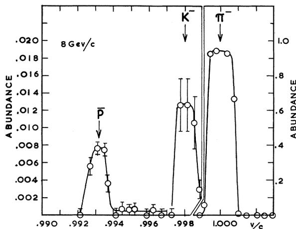
FIG. 2. Velocity spectrum of the negative beam of 8-GeV/c momentum.
