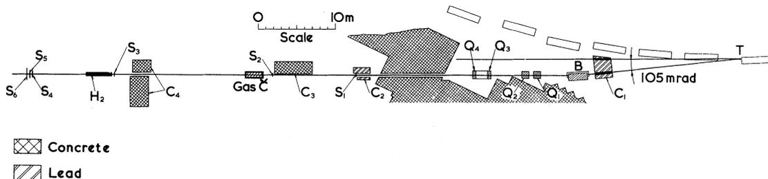
FIG. 1. Experimental layout.  $C_{1-4}$ , collimators;  $B$ , bending magnet;  $Q_{1-4}$ , quadrupole lenses;  $\check{C}$ , gas Čerenkov counter;  $S_{1-6}$ , scintillators;  $T$ , internal target.
