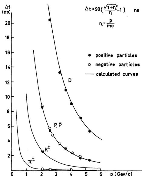
FIG. 5. Time of flight versus momentum for the various particles. The curves are the delays relative to light for a flight path of 27 m, calculated for pions,  $K$  mesons, protons, and deuterons. The experimental points are the average values of the measured delays. The statistical errors are not indicated, as they are smaller than the size of the circles.
