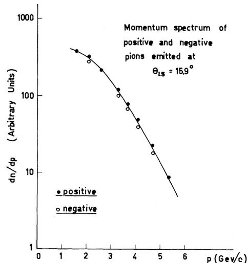
FIG. 4. Momentum spectrum of the pions (slightly contaminated with muons and electrons) emitted at  $15.9^\circ$  from the Al target, and detected at 61 m from it. The spectra at the target can be deduced by correcting for pion decay over the 61-m path.
