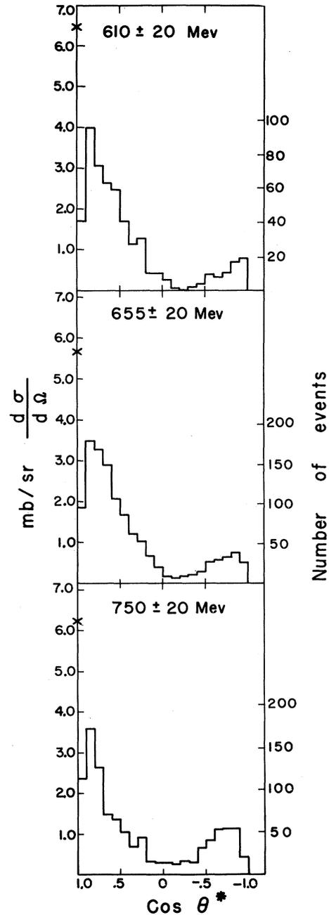
FIG. 2. The elastic scattering angular distributions are given as a function of the cosine of the angle in the center-of-momentum system. The crosses are the predicted forward scattering cross sections.
