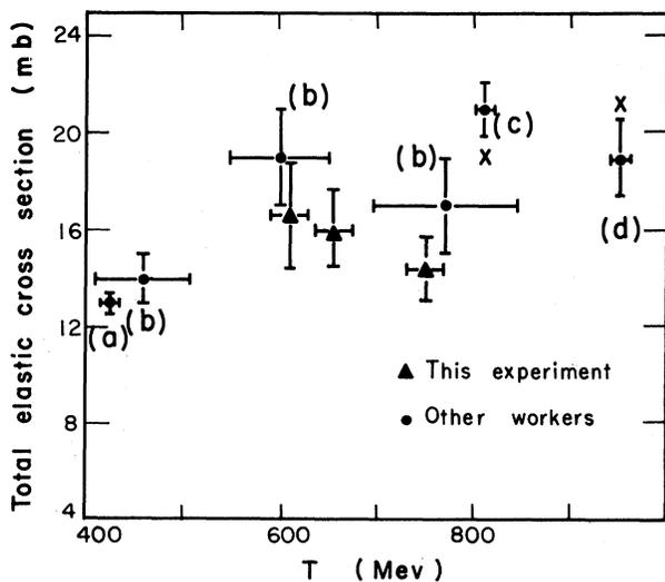
FIG. 1. The total elastic scattering cross section is given as a function of the pion kinetic energy (laboratory system). The crosses show suggested changes in the elastic scattering data based on the latest total cross-section data. (a) Reference 6; (b) reference 7; (c) reference 8; (d) reference 10.
