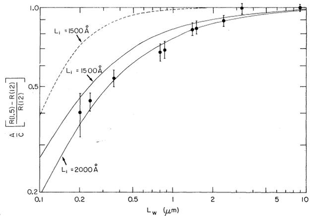
FIG. 4. Normalized resistance rise at 1.5 K as a function of the length of the wire,  $L_w$ . The solid and dashed lines are discussed in the text.
