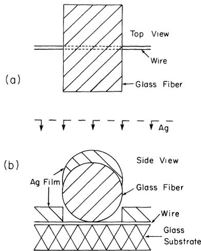
FIG. 1. Description of the method used to make the short wires studied in this work.
