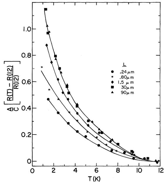
FIG. 2. Normalized resistance rise  $(A/C)[R(T) - R(12 \text{ K})]/R(12 \text{ K})$  as a function of temperature for wires of various lengths. The wires had diameters of 590, 500, 430, 370, and  $600 \text{ \AA}$ , where we have listed the value for the longest wire first, etc.
