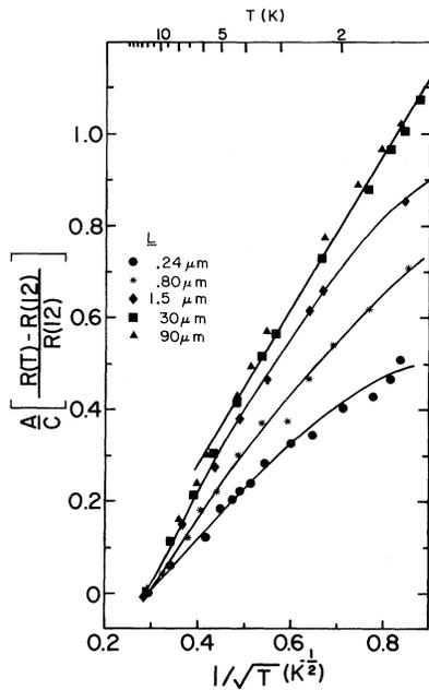
FIG. 3. Normalized resistance rise as a function of  $1/\sqrt{T}$ . Some of the data points have been omitted for clarity. Note that while the results for the 90- $\mu\text{m}$  wire fall slightly above those for the 30- $\mu\text{m}$  sample, this difference is within the uncertainties in the values of  $A$  used in the normalization and is therefore not significant.
