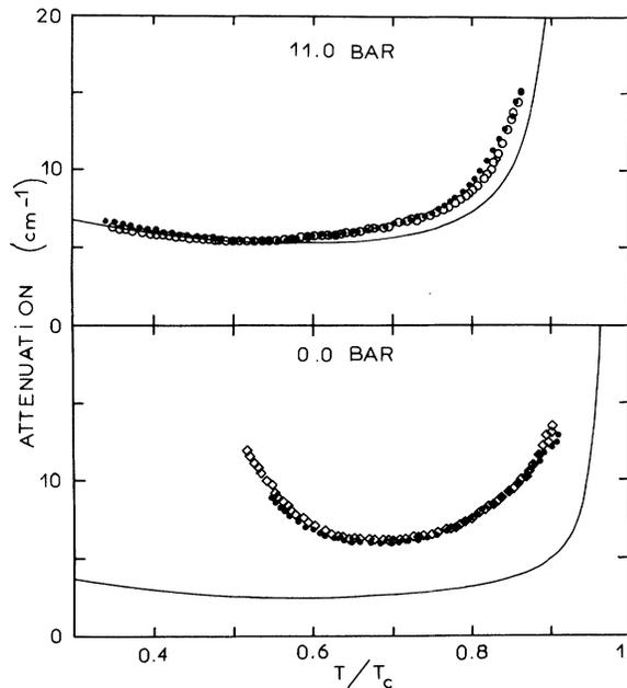
FIG. 1. Amplitude attenuation of zero sound in inverse centimeters vs  $T/T_c$  in superfluid  ${}^3\text{He-A}$  at the pressures of 0.0 bar (bottom) and 11.0 bars (top) for two values of the applied magnetic field (diamonds, 4 kG; open circles, 5 kG; closed circles, 8 kG). The plain curves are the weak-coupling theoretical results obtained from Eqs. (1)–(3), with use of the gap function and the values of the parameters given in Fig. 2 and in its caption.
