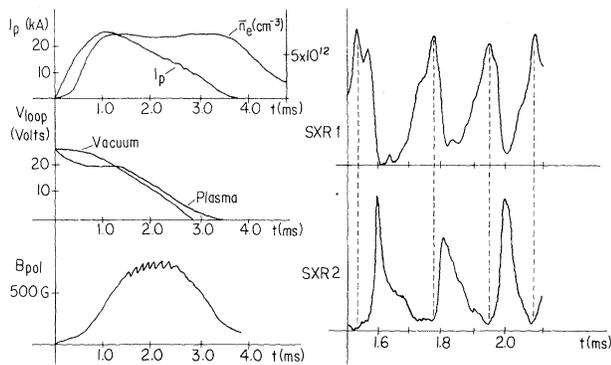
FIG. 2. Typical parameters for low- $q$  discharges. The SXR signals are shown in expanded time scale. SXR1 is the central-chord signal and SXR2 is the signal from the separatrix region that shows the sawtooth inversion. The line-averaged density includes both the central tokamak and scrape-off regions.
