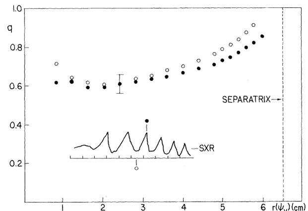
FIG. 4. Time dependence of the  $q$  spatial profile during a sawtooth period. The points corresponding to the sawtooth valley are plotted relative to the minor radius along the midplane, while those for the peak are plotted for the same values of poloidal flux as the valley regardless of the actual radius. An error bar is shown which represents the possible offset of both curves. The possible error in the relative values of peak and valley  $q$  values is estimated to be 25% of the error shown.
