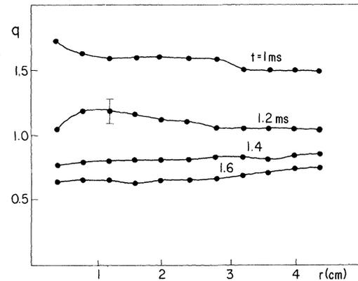
FIG. 3. Approach of the  $q$  profiles to the low- $q$  state.  $q$  is plotted vs the distance from the magnetic axis along the midplane, for a case where  $q$  reaches 0.6.
