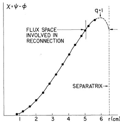
FIG. 5. The helical flux  $\chi$  for a low- $q$  Tokapole II discharge before reconnection. The region of helical flux space which would be involved in the reconnection if the island did not extend beyond the separatrix is shown.
