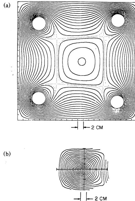
FIG. 1. (a) Theoretical flux plot generated numerically from the Grad-Shafranov equation. The dotted lines represent the separatrices which encircle the plasma and one or more of the divertor coils; the outer boundary represents the conducting wall. (b) Experimental flux plot generated directly from magnetic probe measurements.
