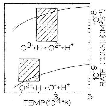
FIG. 3. Theory of Butler, Heil, and Dalgarno (solid line) and experimental results (shaded areas). (The shaded areas represent  $\pm 1$  standard deviation uncertainty.)
