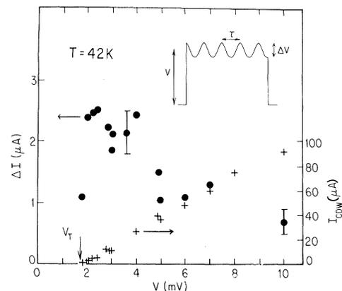
FIG. 1. Amplitude of the current oscillation  $\Delta I$  and CDW current  $I_{CDW}$  vs voltage in NbSe<sub>3</sub>. The threshold voltage  $V_T = 1.75$  mV. The upper portion of the figure is a schematic representation of the response wave form from a current pulse with  $I$  well above  $I_T$  (see Ref. 5).
