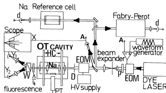
FIG. 1. The experimental arrangement. A, feedback signal; D, diaphragm; d, detector; EOM, Pockels EO modulator; HC, Helmholtz coils;  $\lambda/4$ , quarter wave plate; p, polarizer; PT, phototube; and W, Wollaston prism.
