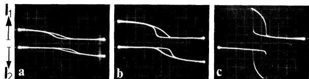
FIG. 3. Hysteresis in the output vs input polarization as the latter is scanned from almost circular polarization to the opposite almost circular polarization, at different light intensities. (a) 5 mW, (b) 20 mW, and (c) 30 mW (both traces partially cut by the scope window).
