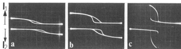
FIG. 3. Hysteresis in the output vs input polarization as the latter is scanned from almost circular polarization to the opposite almost circular polarization, at different light intensities. (a) 5 mW, (b) 20 mW, and (c) 30 mW (both traces partially cut by the scope window).
