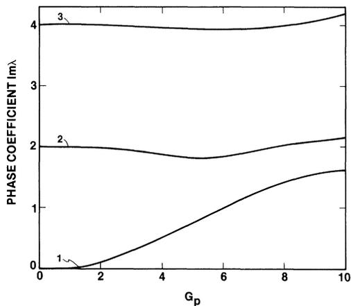
FIG. 2. Imaginary parts of eigenvalues vs plane-wave gain coefficient,  $G_p$ , for  $\mu = 0.5$ .
