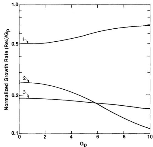
FIG. 1. Normalized real parts of eigenvalues vs plane-wave gain coefficient  $G_p$ , for  $\mu = 0.5$ .
