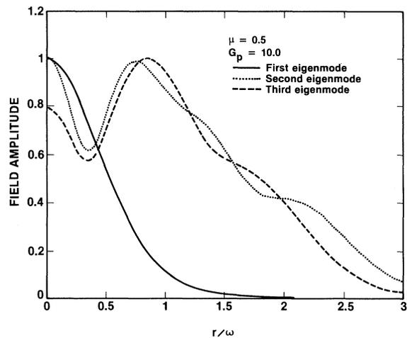
FIG. 3. Magnitudes of eigenmode fields vs normalized radial coordinate.
