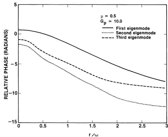
FIG. 4. Eigenmode phase deviations from free-space mode curvature vs normalized radial coordinate.
