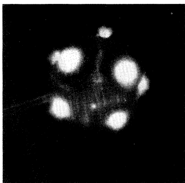
FIG. 4. X-ray pinhole photograph of energy deposition in a 300- \mu\text{m} -diam gold sphere irradiated symmetrically with eight beams.
