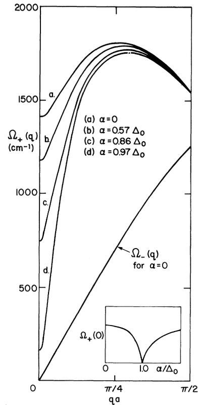
FIG. 2. The phonon spectrum as a function of  $\alpha$ . The acoustic branch is only weakly dependent on  $\alpha$ .
