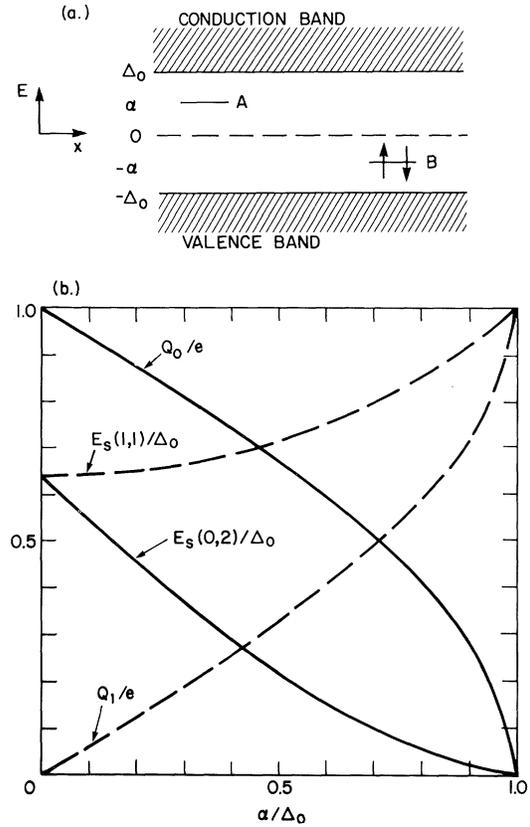
FIG. 3. (a) Formation of the (lowest-lying)  $AB$  soliton pair (schematic), and (b) the charges and excitation energies of the spin-0 and spin- $\frac{1}{2}$  solitons (see text).
