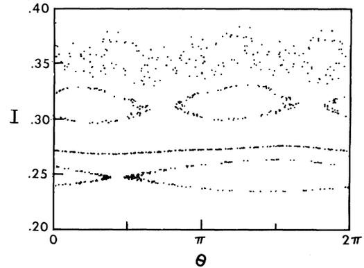
FIG. 1. Island chains for the  $m = 1, 2, 3$  resonances for a perturbation with  $\Omega = 1$  and  $\epsilon = 0.00375$ . The  $m = 3$  islands already exhibit large stochastic regions. Also shown is a confining KAM surface between the  $m = 1$  and  $m = 2$  resonances.
