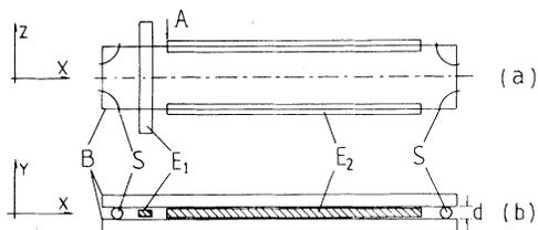
FIG. 1. A sketch of the liquid-crystal cell.
