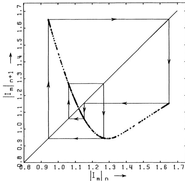
FIG. 3. The one-dimensional mapping function  $|I_m|_{n+1}$  vs  $|I_m|_n$  (in units of  $V_f/R$ ) for the 744th through the 999th cycle for  $V_0/V_f = 18$  in the chaotic region. The circuit parameters in this case were  $\omega = \omega_0$ ,  $Q = 15$ ,  $\tau_m = 2\pi/\omega$ , and  $I_c R/V_f = 2.0$ .
