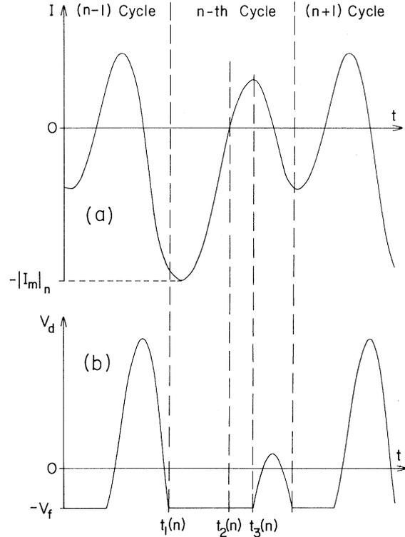
FIG. 2. Typical response of the driven diode resonator calculated with use of the model described in the text. The response for the case shown has a period twice that of the drive period. The times  $t_i(n)$  which determine the  $n$ th cycle are described in the text. (a) Current vs time for three consecutive cycles. (b) Voltage across the diode vs time.
