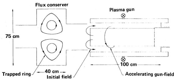
FIG. 1. The Beta II plasma gun experiment (Ref. 7) shown schematically. The initial field is established, D<sub>2</sub> gas is puffed in, and the gun is fired. Plasma with embedded acceleration gun field emerges from the gun stretching the initial field into the flux conserver. Reconnection of the field produces an isolated trapped ring.
