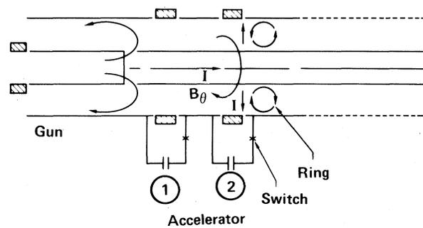
FIG. 3. An extended gun accelerator. Here a ring is produced as described in Fig. 1 and accelerated by  $B_\theta$  field injected behind the ring by successively firing accelerator banks 1, 2, etc. Current flows in the center conductor as indicated and returns radially at the interface of the accelerating  $B_\theta$  and ring field and through the gun and accelerator capacitor banks. It is assumed that sufficient plasma is present at the interface to support current flow.
