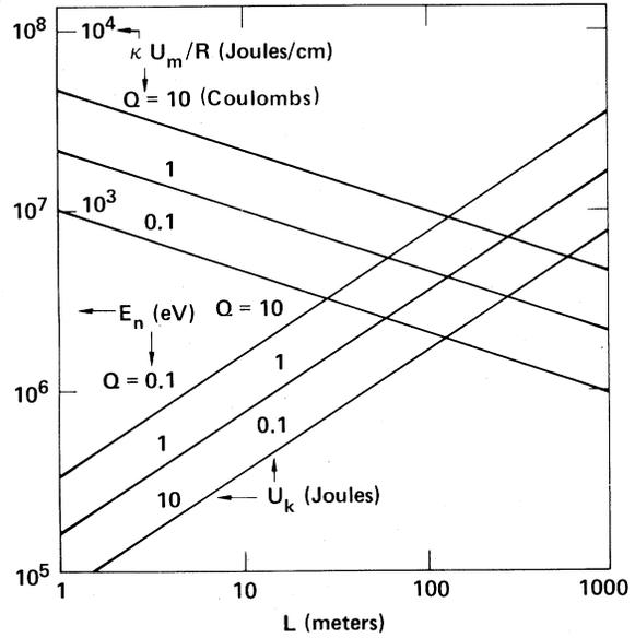
FIG. 2. Ring kinetic energy  $U_k$ , energy per nucleon  $E_n = U_k/Q$ , and ring magnetic energy divided by radius  $\kappa U_m/R$  vs accelerator length  $L$  for several values of  $Q$ . Here the maximum power delivered to the ring is held constant at  $P_r = 10^{12}$  W, and  $Q = eM_r/m_p$ . The quantities  $\kappa$  and  $P_r$  are defined in the text.
