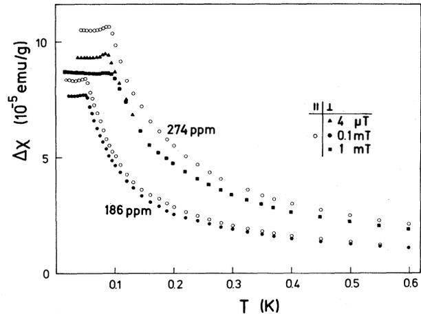
FIG. 3. Magnetic susceptibility  $\Delta\chi(T)$  for two MgMn single crystals as measured parallel and perpendicular to the  $c$  axis.
