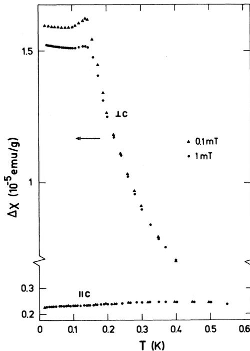
FIG. 2. Magnetic susceptibility  $\Delta\chi(T)$  for a CdMn single crystal as measured in different fields parallel and perpendicular to the  $c$  axis.
