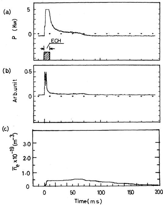
FIG. 3. (a) Bolometer signal, (b) spectral line signal of C III, and (c) line-averaged electron density vs time.
