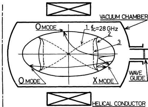
FIG. 1. Experimental configuration. 1: Resonance surfaces of  $f_c = 28$  GHz ( $B = 1$  T). 2: Right-hand cut-off. 3: Upper hybrid cutoff. Ray tracings of ordinary (O) mode and extraordinary (X) mode are indicated by solid lines.
