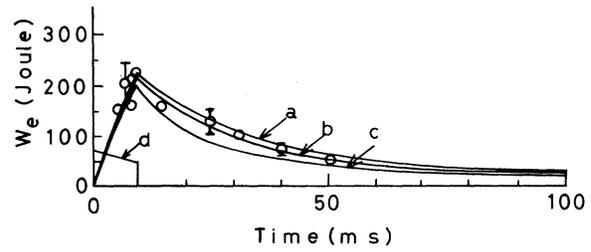
FIG. 4. Total electron energy  $W_e$  vs time. The solid lines are total electron energies calculated from transport code with different values of anomaly factor  $C$ : Curve  $a$ ,  $C = 1$ ; curve  $b$ ,  $C = 3$ ; and curve  $c$ ,  $C = 10$ . Curve  $d$  is the rf power used in the calculation. The power is 70 kW at  $t = 0$  and 50 kW at  $t = 10$  msec.
