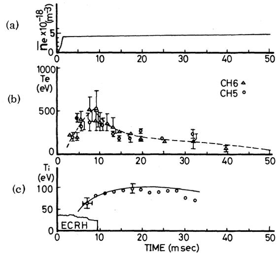
FIG. 2. (a) Line-averaged electron density, (b) central electron temperature, and (c) ion temperature vs time. The solid line is ion temperature calculated from neoclassical transport code.
