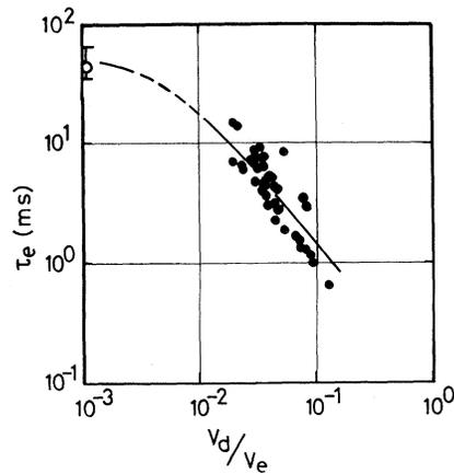
FIG. 5. Electron energy containment times vs the drift parameter  $V_D/V_e$ . Results from Ohmically heated plasmas are given by filled circles and that from the ECRH plasma is given by an open circle.
