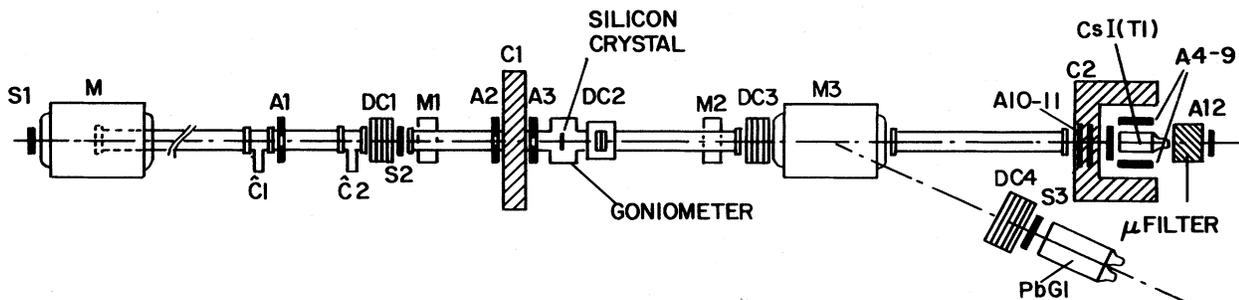
FIG. 1. Experimental apparatus. S1-S4 are the trigger counters while A1-A12 are the vetoes. DC1-DC4 are drift-chamber modules. M and M1-M3 are magnets for calibration and background elimination. C1 and C2 are threshold Cherenkov counters.
