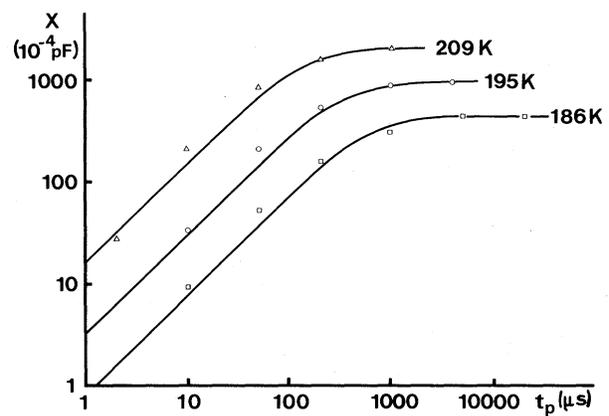
FIG. 3. Amplitude of the DLTS signal  $X$  (G2) as a function of pulse width  $t_p$  at various temperatures (logarithmic scale). Full lines are empirical fits with the law  $X = X_0 [1 - \exp(-c_n t_p)]$ . The shift in the saturation amplitude as the temperature increases is explained by the effect of the sample series resistance.
