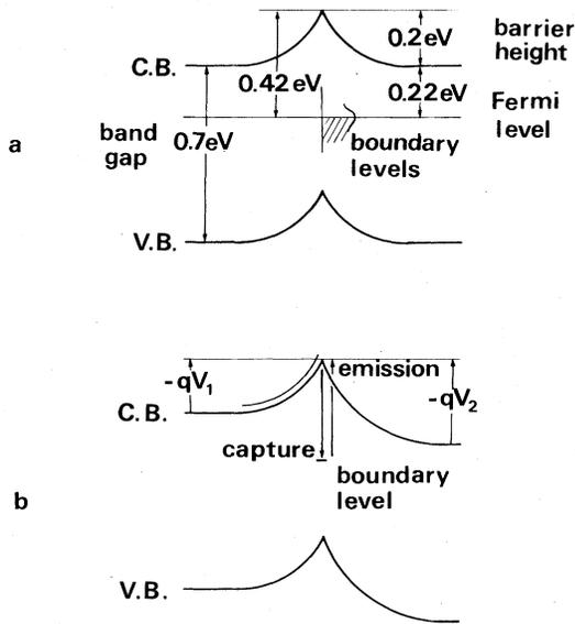
FIG. 1. Band bending near a grain boundary (a) at thermodynamic equilibrium and (b) under bias. The numerical values are justified in the text.
