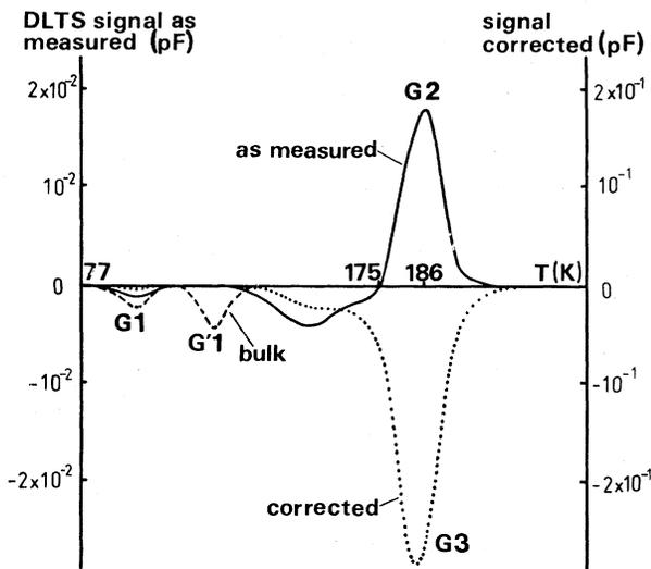
FIG. 2. Boundary spectrum as measured (full line) with pulse rate  $10 \text{ s}^{-1}$ , pulse width  $200 \mu\text{s}$ , and pulse height  $0.5 \text{ eV}$ , and after correction for the sample series resistance effect (dotted line) and bulk trap spectrum (dashed line). The peak G'1 ( $0.38 \text{ eV}$ ) is observed in the bulk spectrum only. It could be associated with the acceptor level of copper (Ref. 14) diffused in the process of making the Schottky diode.
